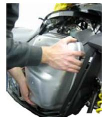
Gently pull muffler back, up, and out.
