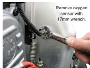
Remove oxygen sensor with 17mm wrench.
