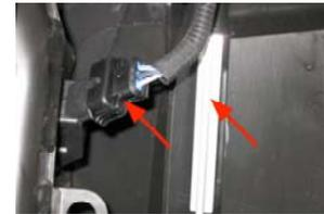
Remove both slide clips and unplug air volume sensor.
