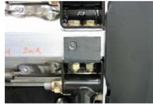
6.) DRILL OUT SIX RIVETS holding plastic under panels to chassis (3 on each side). Using a 1/4" drill bit, drill out the 6 rivets shown in picture below. You may need to hold back of rivet with a small vise grip to keep it from spinning while drilling.
