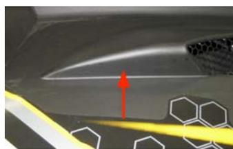
Rear section of air scoop pushes up against rear of plastic body panel air duct.
