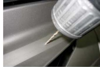
Drill pilot holes, then final hole size.
