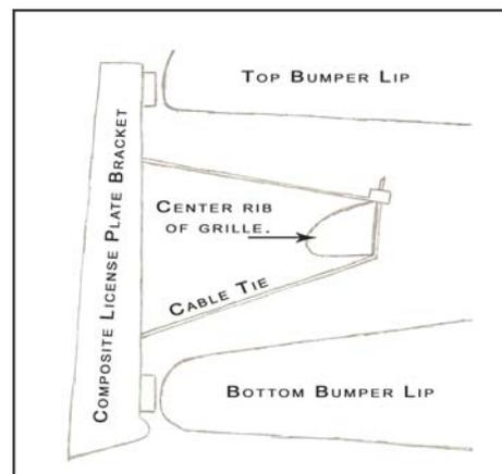
3. Feed pre-bent cable ties through the holes on the backside of the Plate Bracket. The cable tie cam should be in the top hole position as shown in the previous illustration and photo to the right.
